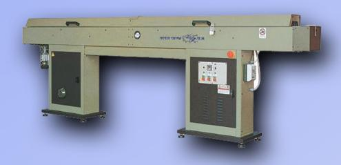
The machine has been innovated with new technology. It is widely used for drying the dyed edges of belts, bags straps, welts and strips for interwoven products. Due to its characteristics, it can be included in automated production cycles. The dried products are not altered in any way. The machine is provided with safety protections in compliance with regulations in force.
