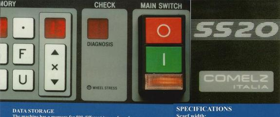
The machine has a memory for 800 different types of scarf (100 groups of 8) and each one is immediately accessible. It is sufficient to press a button to recall the required type of scarf.
